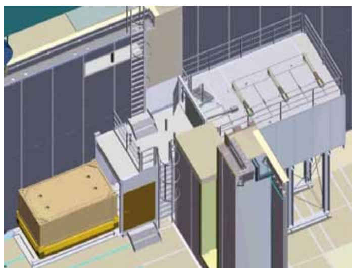
Packaging station with transfer, sealing and loading areas (from left to right)
